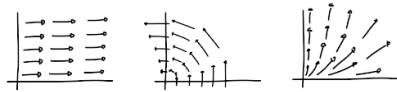
Figure 1.5: The flow fields to the translation symmetry, the rotation symmetry and the scale squish symmetry from left to right.
